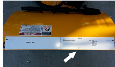
2) Place plow in front of snow blower make sure it's place equally from both sides. Take template that has been provided for you, place it at the edge & middle of the housing and mark your holes.
