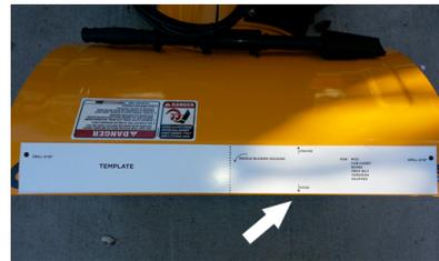
2) Place plow in front of snow blower make sure it's place equally from both sides. Take template that has been provided for you, place it at the edge & middle of the housing and mark your holes.
